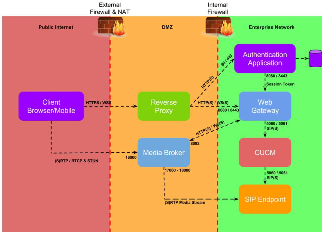
All communications between WebRTC Clients and FCSDK are secure. The Media DTLS handshake will be covered in more detail, but this prevents packet inspection; however, some important details can be gleaned. By default SIP side transactions and media are not encrypted, so more inspection can be performed.
